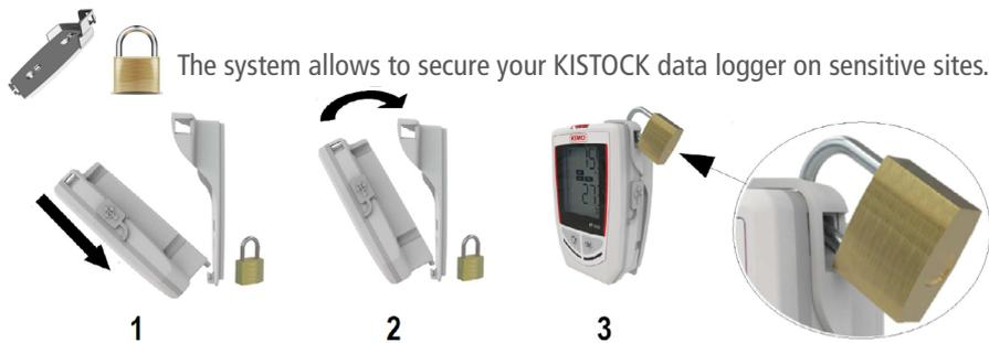
Mount the safety lock support on the required place.
